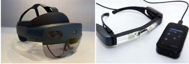
Figure 6. OST AR glasses; left: the Microsoft HoloLens 2. Right: the Epson Moverio BT-40 and the Epson Android base controller BO-IC400.
