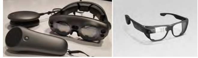
Figure 7. OST AR glasses; left: Magic Leap 1 with the LightPac computing core and the controller. Right: the Epson Moverio BT-40 and the Epson Android base controller BO-IC400.
