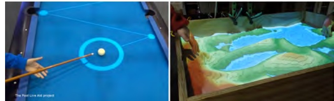
Figure 3. SAR examples: the Pool Live Aid project visualize the redirected path of a billiard ball on the table (left), and the Sand-box project provides an interactive topographic contour line visualization in a sand-box (right).
