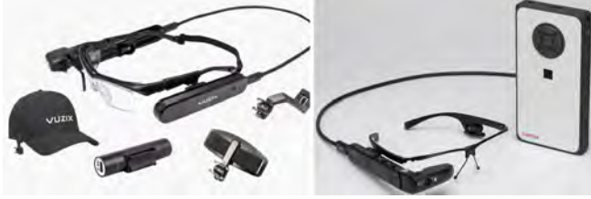
Figure 8. OST AR glasses: Vuzix M4000 with its extra accessories dark shades, battery pack and mountable hat (left), and Toshiba dynaEdge glasses with the dynaEdge DE-100 miniature PC (right).
