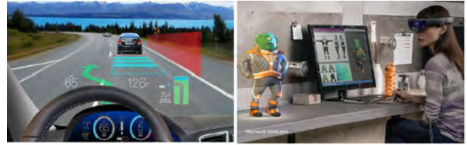
Figure 2. OST AR examples: car heads-up-display which shows the road information (left), and an illustration of how Microsoft HoloLens projects the virtual objects onto the real world (right).
