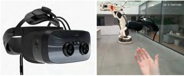
Figure 4. Varjo XR-3 HMD; left: the device. Right: an example AR project captured from XR-3 display.
