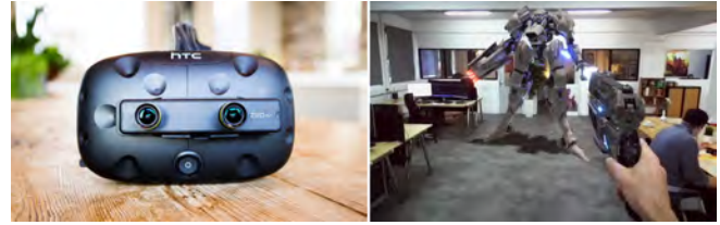
Figure 5. ZED Mini Camera; left: the camera is mounted on a HTC Vive VR headset. Right: an example project created by the Zed Mini which turns the room into a battlefield.
